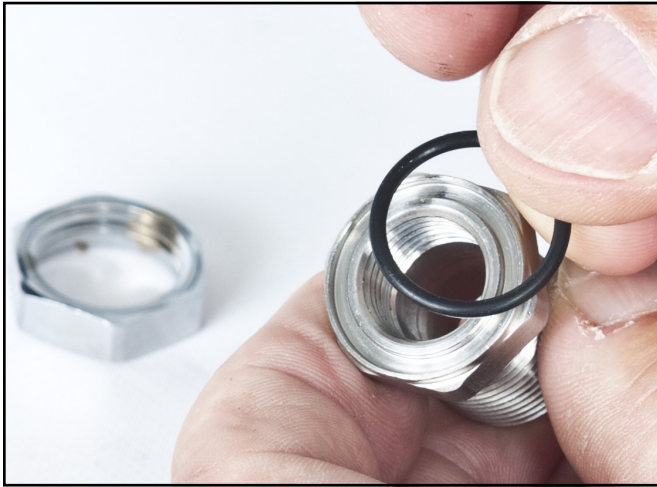
Install the O-ring in the bent tube adapter.
