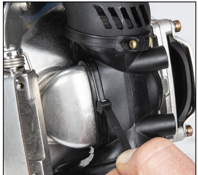
Secure and seal with a tie wrap.
