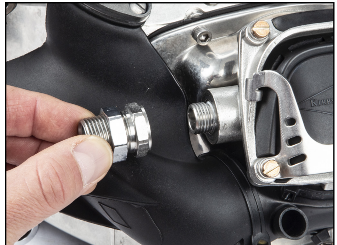
Remove the bent tube adapter.
