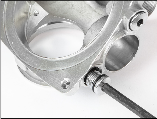
Remove the two port plugs and their O-rings and replace.
