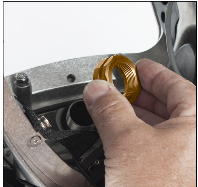
Install the regulator mount nut. DO NOT FULLY TIGHTEN THE NUT AT THIS TIME.
