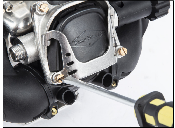
Loosen the screws and washers on either side of the cover.
