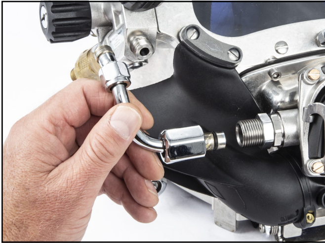
Remove the bent tube assembly.
