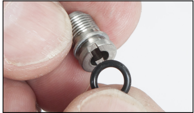
Install the O-ring on the inlet nipple.
