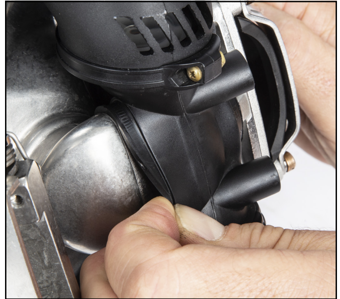
Insert the tube on the exhaust main body onto the tube of the helmet pod.
