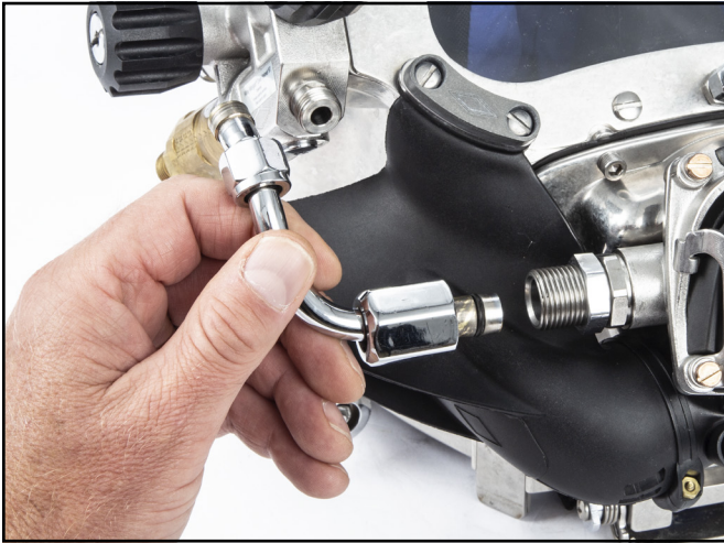
Install the bent tube assembly.
