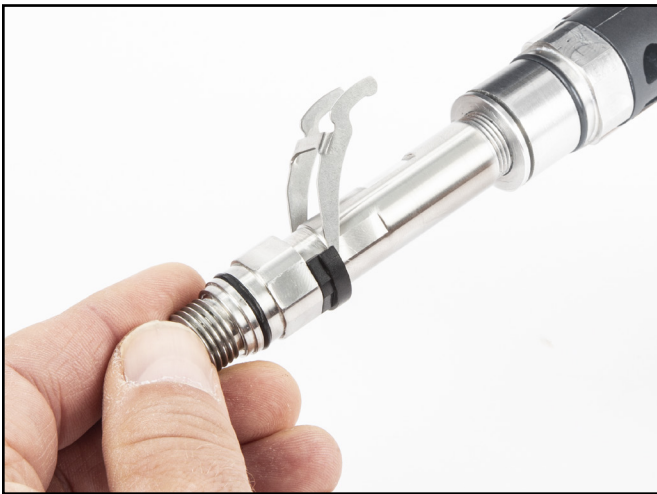
Install the bearing clip onto the outside of the main tube.
