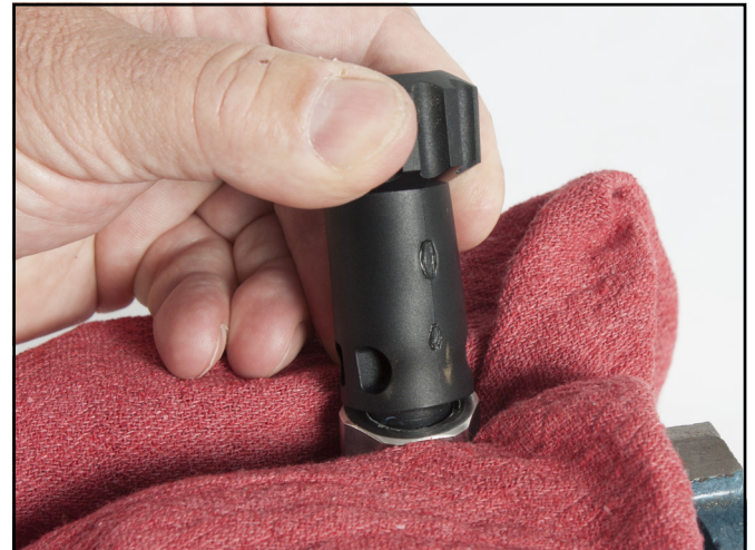
Place the packing nut into a vise and insert the flex knob into the adjustment packing nut at an angle.
