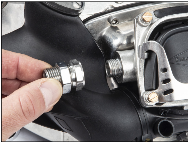
Remove the bent tube adapter and O-ring.
