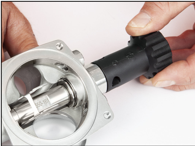
Turn in on the flex knob until an audible click is heard then out three full turns.
