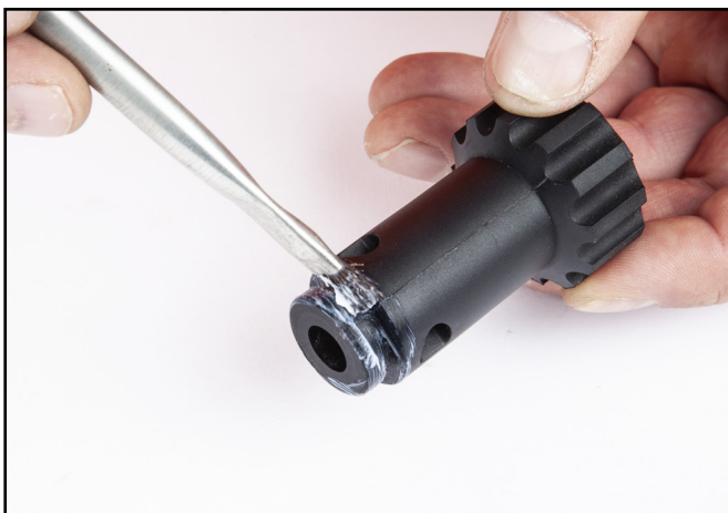
Lightly lubricate the groove in the end of the flex knob.
