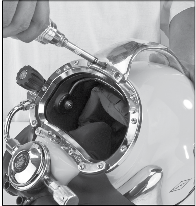
Use a torque screwdriver to tighten the front handle. See "Torque Specs" module.
