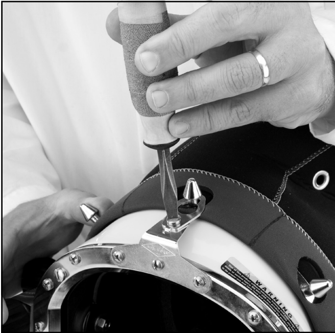
Tightening the top band keeper.
