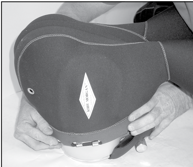
Mount the hood and bands on the mask frame.
