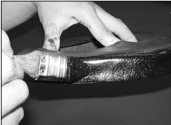
Apply glue to the outer edge of the new face seal.
