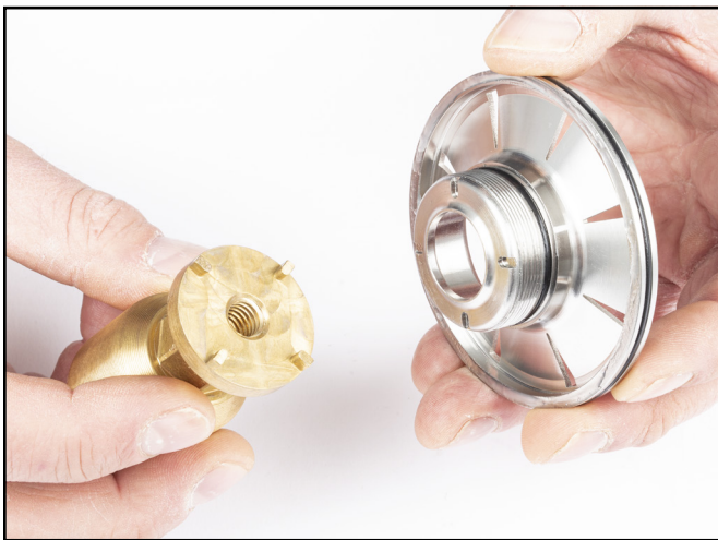
7. Thread the BLACK tool handle into the brass removal tool.
