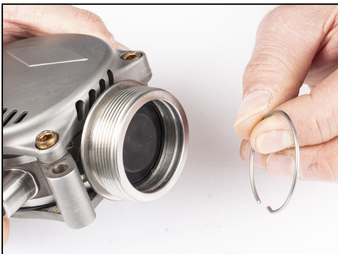
5. Insert Retainer Ring into OPRV body.
