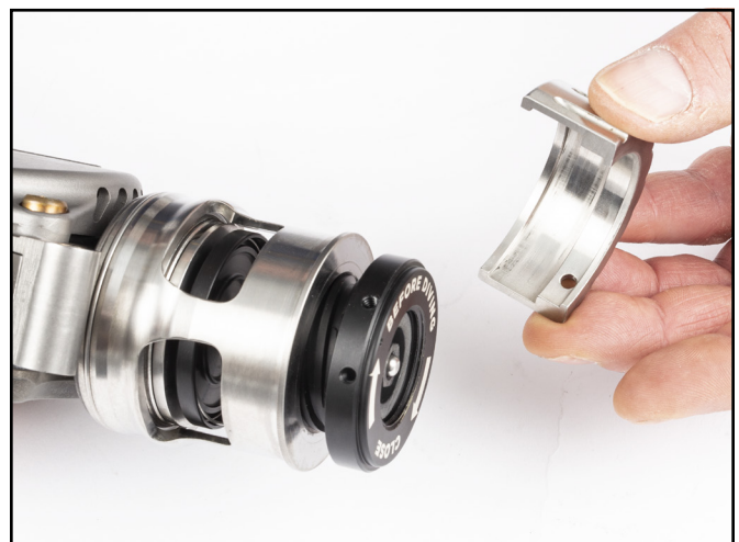
14. Tighten hex screws until the top of the screw is just barely below the outer surface of the knob.
