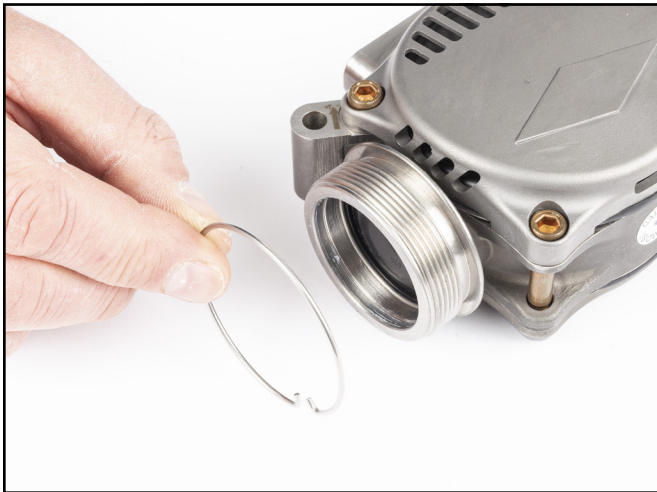
14. Remove OPRV components from Diamond Exhaust body. Use jeweler's type screwdriver to remove Retaining Ring first.
