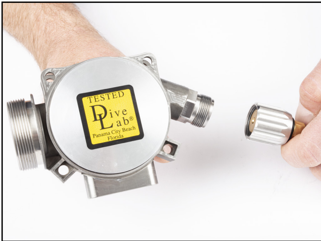
4. Positive pressure test for 10 seconds @ 5 PSI - NO loss of pressure equals a pass on the pressure test.
