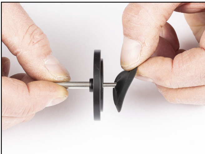
7. Remove valve from puck assembly.
