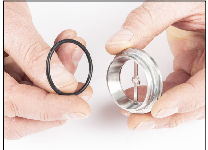
7. Insert the puck seal with O-ring evenly into the exhaust valve body, and push in EVENLY until completely seated.
