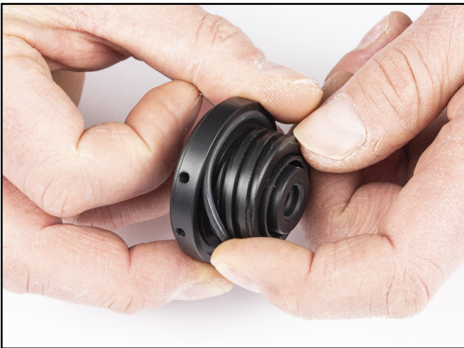
10. Be sure to remove O-ring that is pressed into the Exhaust Control Body.
