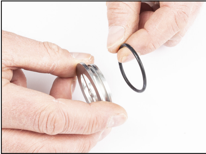
13. Remove Housing Retainer Ring.
