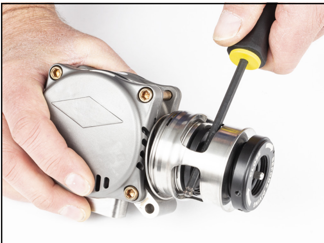
13. Place Split Retainer onto control Control Knob, aligning the holes.
