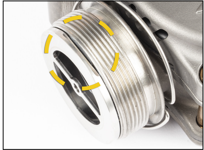
11. Use a large flat blade screwdriver and remove with an even pull outward alternating between sides to pry loose evenly.
