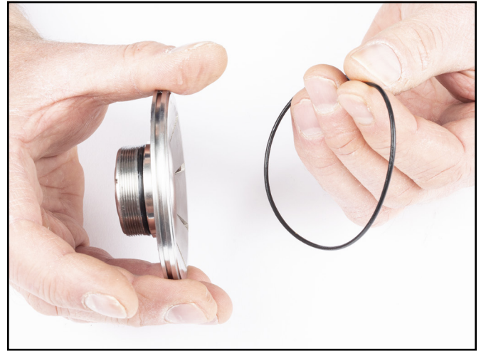
9. Carefully use a pic to remove smaller O-ring.
