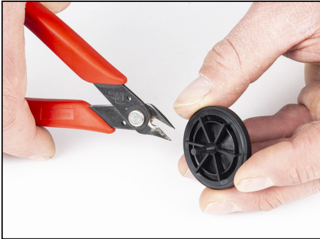
4. Install Exhaust Valve Insert with valve into OPRV body.
