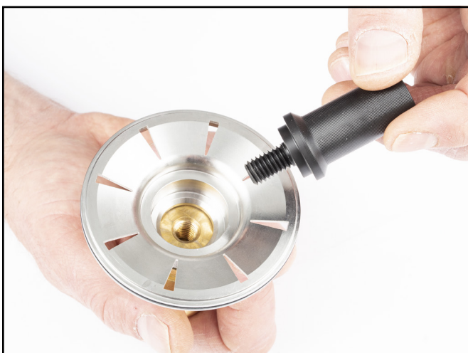
7. Thread the BLACK tool handle into the brass removal tool.
