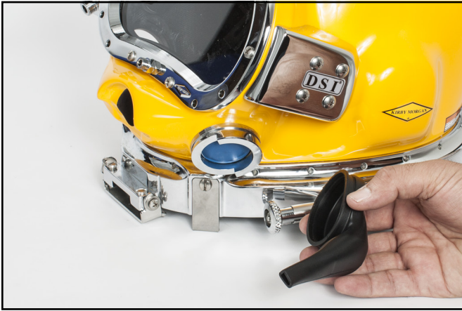
The water purge deflector is removed by cutting the tie wrap that holds it in place.
