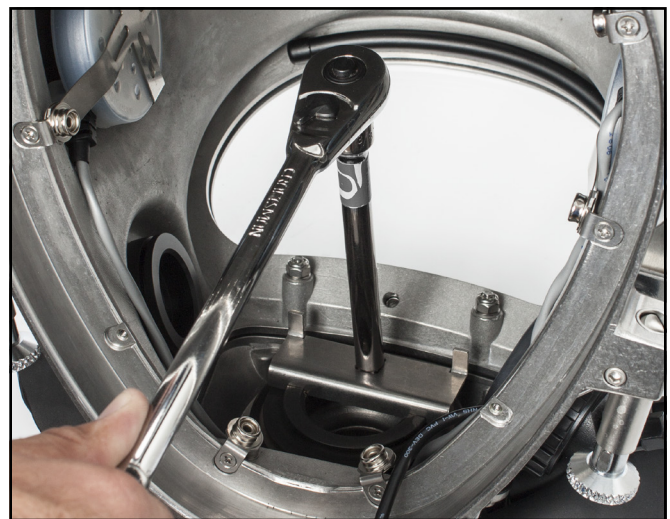
Loosen the regulator mount nut to make it easier to remove the pod.
