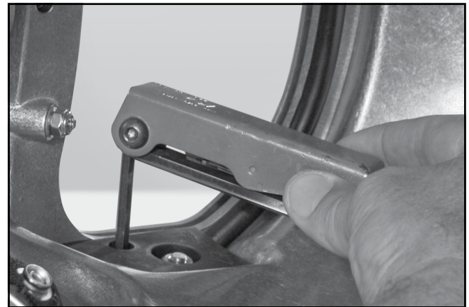
Remove the alignment stud from within the air train body.
