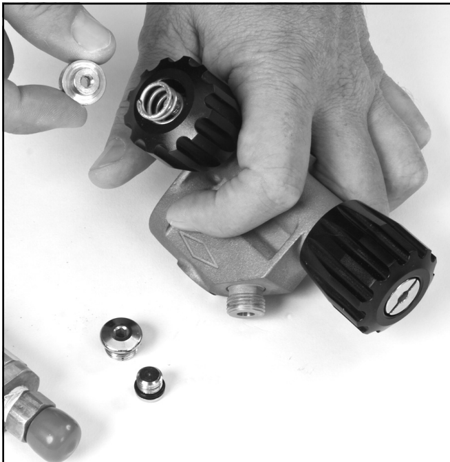
Remove the lock nut and spring
