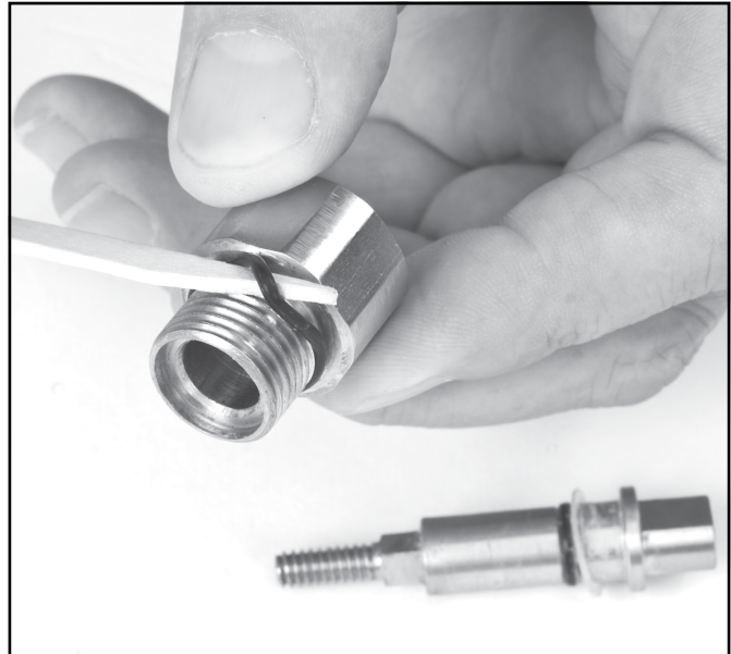
Use a toothpick, credit card, or other non-metal objects to remove the O-rings for cleaning and replacement. Note that the bonnet on the EGS valve is shorter than the bonnet on the steady flow valve.
