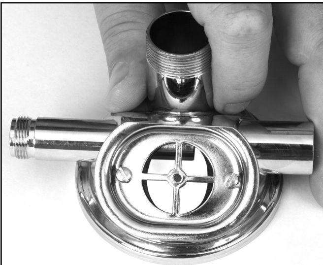
If the flange is tightened too much, the gasket will protrude into the exhaust valve opening and interfere with proper regulator performance.
