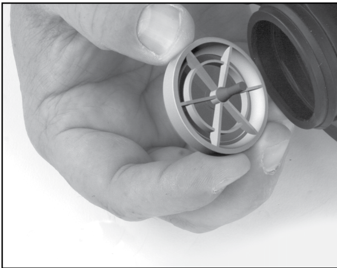
Inspect the exhaust valves on a regular basis.
