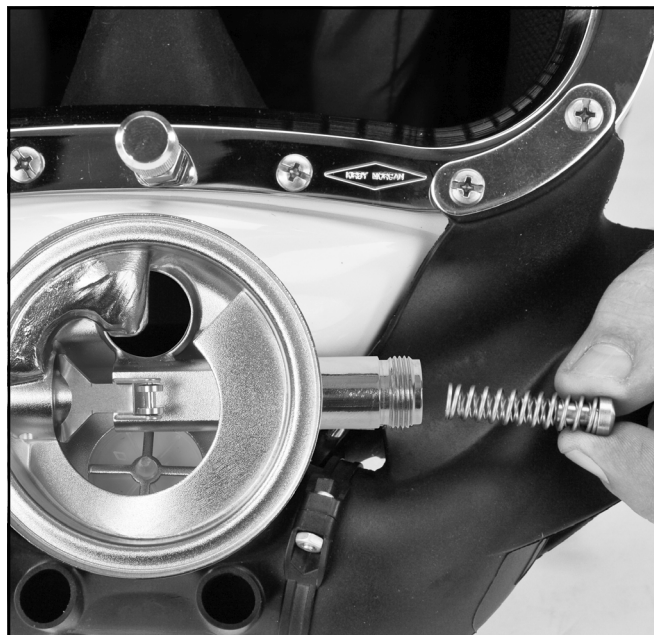
Shake out the spacer, spring set, and piston
