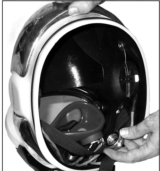
Remove the mount nut from the regulator.
