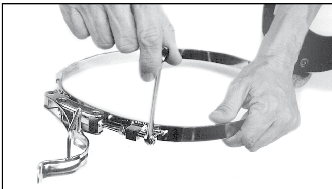
The neck clamp and latch catch must operate properly. They must be regularly inspected and serviced.
