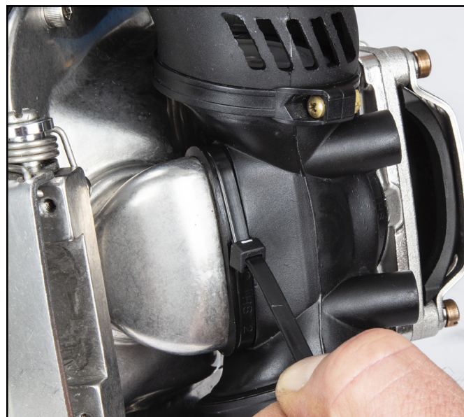
Secure and seal with a tie wrap.
