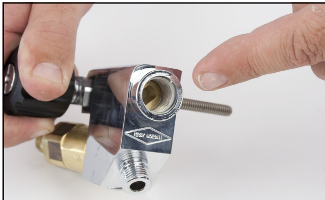
The seat should be removed for inspection.
