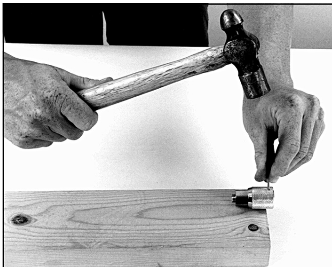
Install the retaining pin into the adjustment knob.
