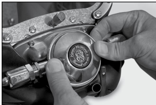
Press the cover over the diaphragm.
