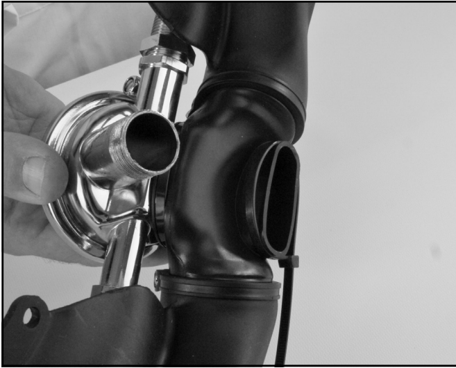
Pre-install the tie wrap.
