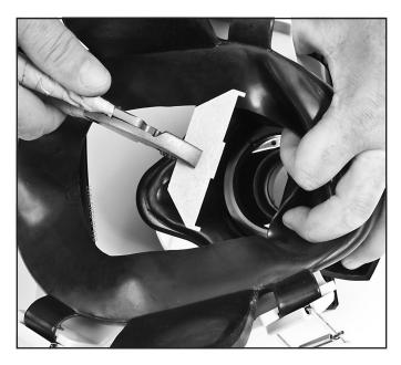
Pliers can also be used to grip and turn the regulator removal tool.
