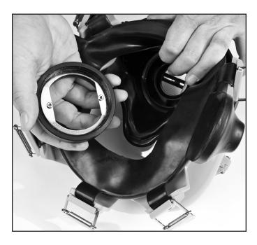
To remove the regulator, you must remove the regulator mount nut.
