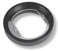
Cross threading can damage the regulator body. If the threads are damaged in any way the body must be replaced. Once the mount nut is on correctly, start tightening. Once again, check and make sure that the exhaust whisker is properly seated in the frame before final tightening. Tighten the regulator mount nut to 100 inch pounds.
