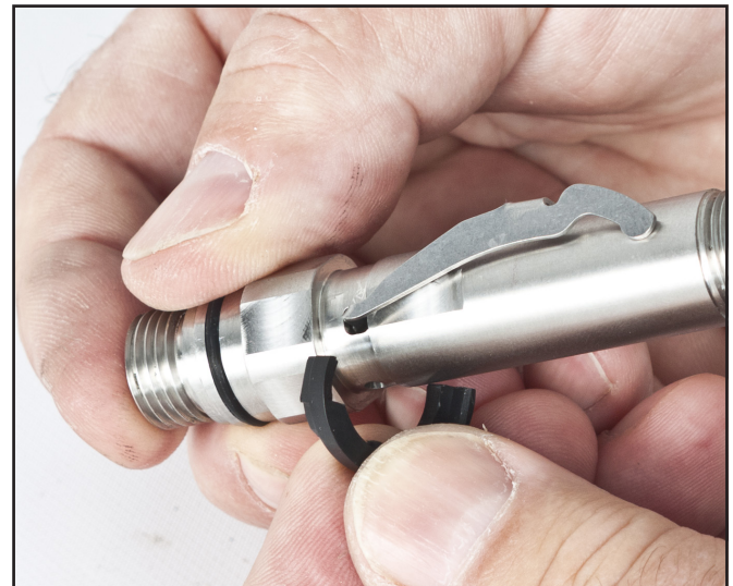
Remove the bearing clip.
