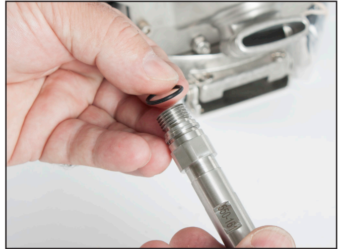
Remove the O-ring from the main tube.
