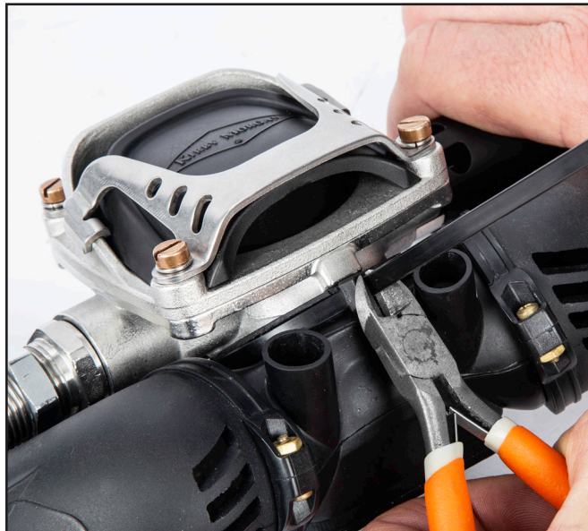
Remove excess tie wrap.
