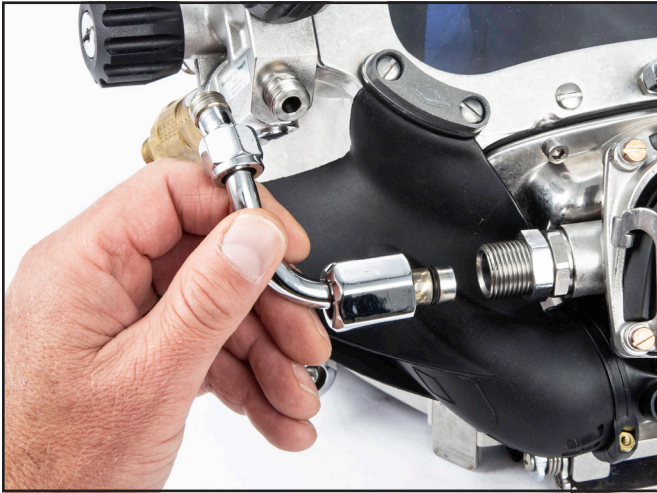
Remove the bent tube assembly.
