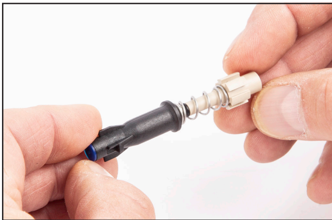
Using the balance spacer with the two O-rings installed, insert the first O-ring into the open end of the inlet valve and stop.
