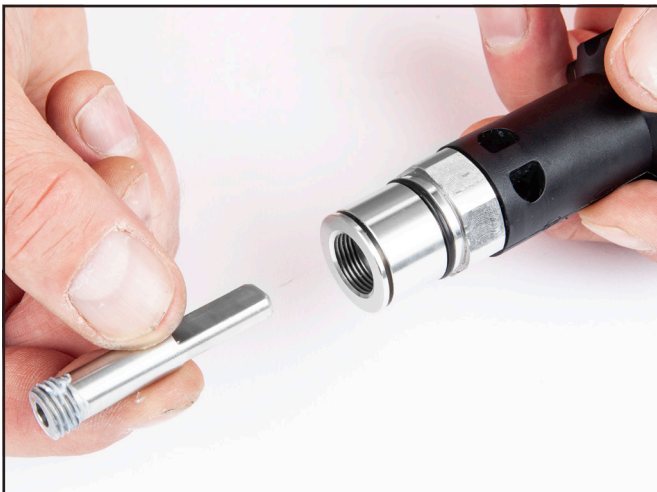
Lubricate the threads of the adjustment
