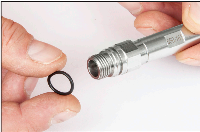
Install the O-ring onto the main tube.
