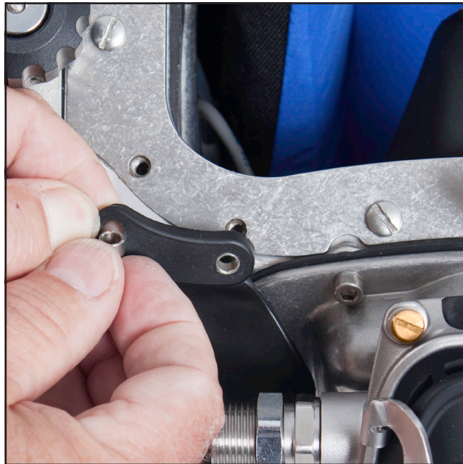
Attach the whisker to each side of the face port retainer using the spacers, zinc anodes or kidney plates and screws.
