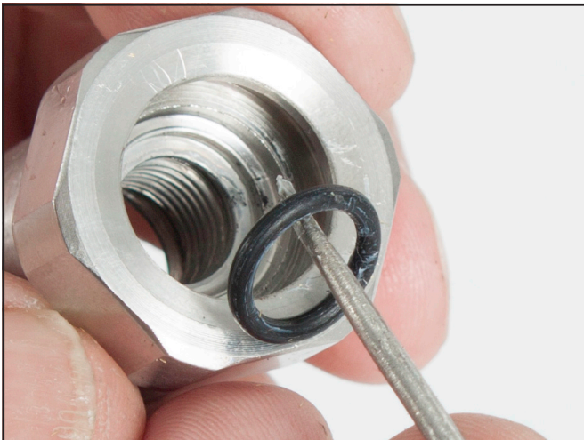
Using an O-ring pic, carefully remove the bearing washer and adjustment shaft O-ring.
