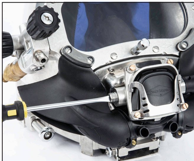
Turn the adjustment nipple ¼ of a turn at a time to adjust the performance of the regulator.
