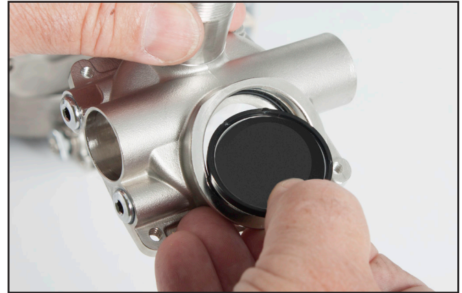
Install the O-ring and valve insert.
