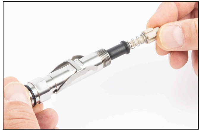
Align and insert the inlet valve into the main tube.
