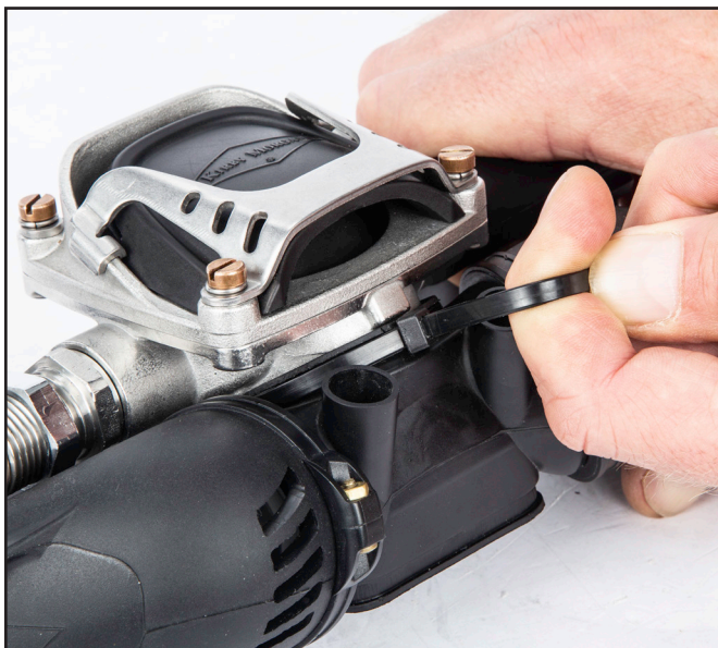
Install the tie wrap on the regulator.
