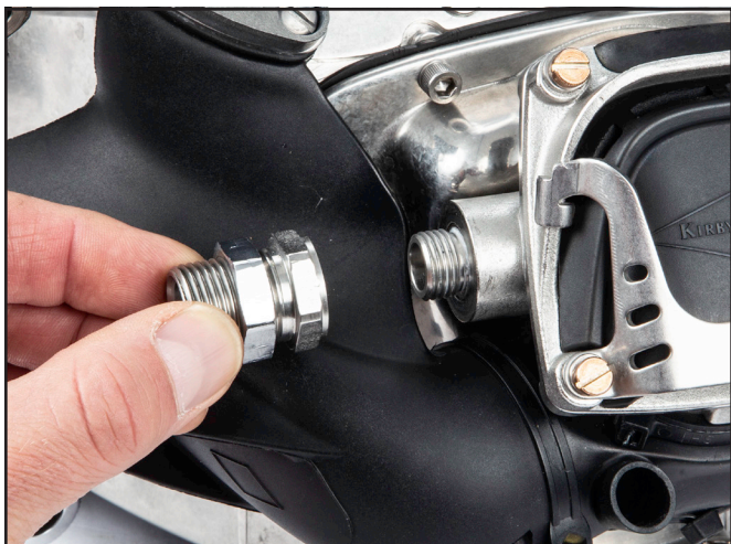
Remove the bent tube adapter.
