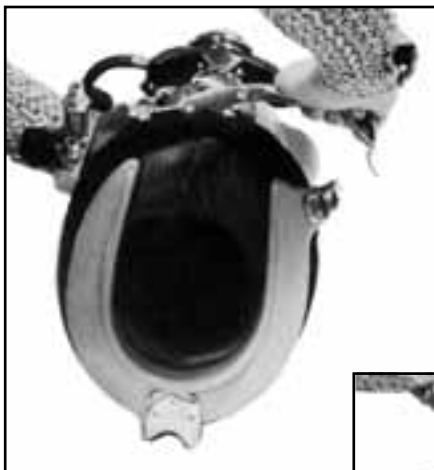
Fig. 2 The yoke hinges open showing the rubber neck dam. The neck dam is always turned up as shown. Overpressure on the interior of the hat pushes outward on the neck dam, but the yoke prevents ballooning.
