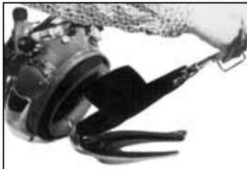
Fig. 2 The yoke hinges open showing the rubber neck dam. The neck dam is always turned up as shown. Overpressure on the interior of the hat pushes outward on the neck dam, but the yoke prevents ballooning.
