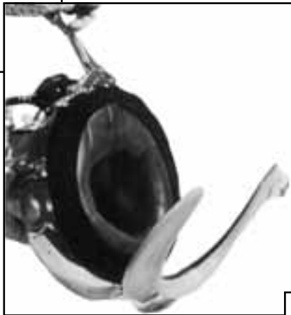
Fig.3 The neck dam/yoke system is removed completely from the helmet.
