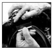
3. Place swing catch P/N 545-077 in position on neck ring. Bent edge of catch should face in.
