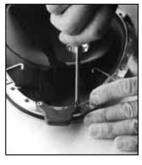
8. Use the two small Phillips screws to attach tongue spacer to underside of neck step ring. (Tongue catches on older neck rings may be too long and will need to be trimmed to match the new tongue spacer.)
