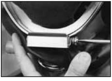
7. Finish tightening screws. Swing catch should close freely and securely with spring pressure.
