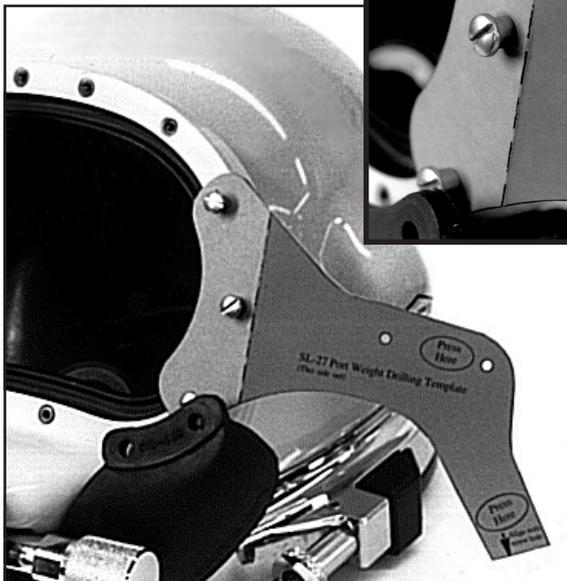
Note: Once the port weight is installed, the chin weight becomes optional depending on the accessories mounted to the helmet.
