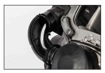
15) Line up the detail features of water tubes A & B, with the mating details of both adapter sleeves.
