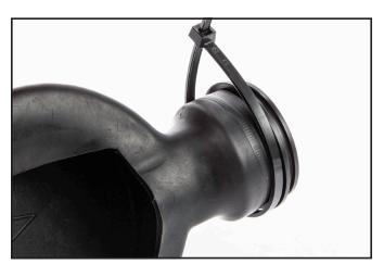
10) Using the narrow tie wrap P/N 520-049, secure sleeve to shroud. Ensure the leading edge of the shroud is pushed flush to the edge of the upraised channel found on the adapter sleeve.
