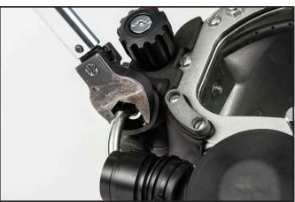
13) Line up the bent tube mount nut to the side block. Complete installation of bent tube assembly. Refer to "1.2.3 Installation of the Bent Tube Assembly" on page BNT-2 from the KMDSI modular manual.
