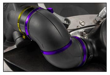
16) Using the narrower tie wrap, P/N 520-049, (represented by the gold color in the photo), secure the long adapter sleeve to the side block shroud.
