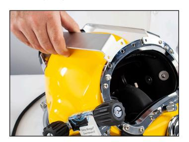
4) Align the holes in the front part of the brackets with the holes in the port retainer. Install one screw in each bracket in the outer mount holes. (Screw P/N 530-040 supplied in the kit) **DO NOT TIGHTEN.**
