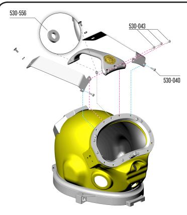
5) Position the handle on the helmet and align all the holes. Install new screws P/N 530-043. First install the 2 outer screws, but **DO NOT TIGHTEN**. Slide the washer P/N 530-556 between the handle and the port retainer and install the center handle screw through the washer. **DO NOT TIGHTEN**.
