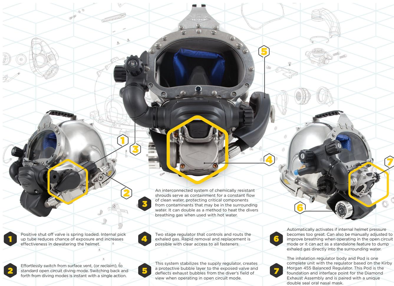
**1** Positive shut off valve is spring loaded. Internal pick up tube reduces chance of exposure and increases effectiveness in dewatering the helmet.
