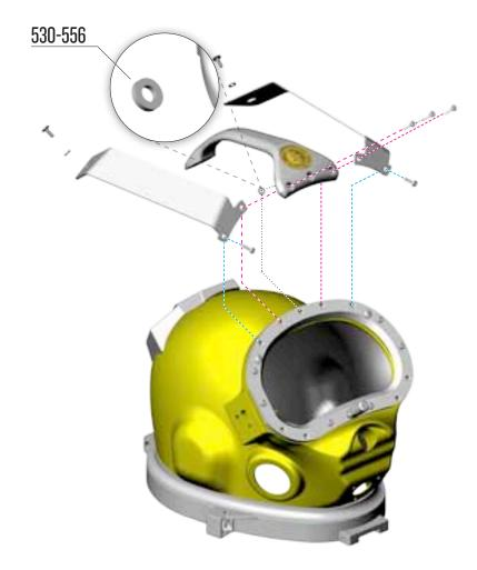
*Above: Detail of the added P/N 530-556 washer's location, behind the front center hole of the handle.*
