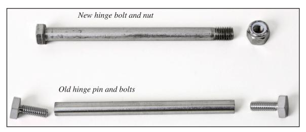
Kirby Morgan Dive Systems, Inc. has simplified the design the hinge pins on all of the KMDSI helmets with the introduction of the hinge bolt (530-027) and lock nut (530-028). This design replaces the previously used pin (550-275) and bolts (530-200).
