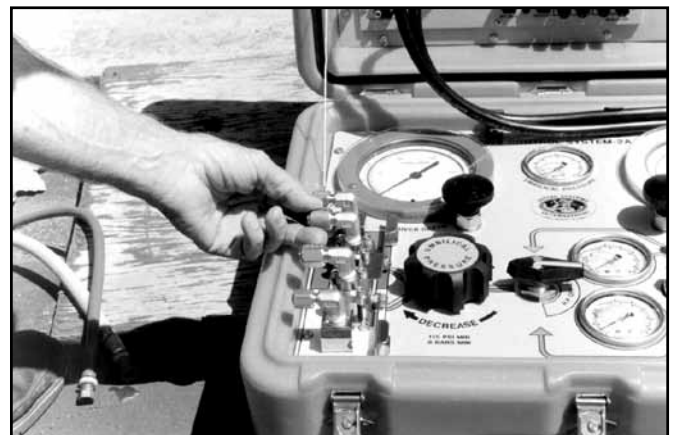
Figure 10 All of the outlet fittings on the KMACS 5 must be capped prior to storage.
