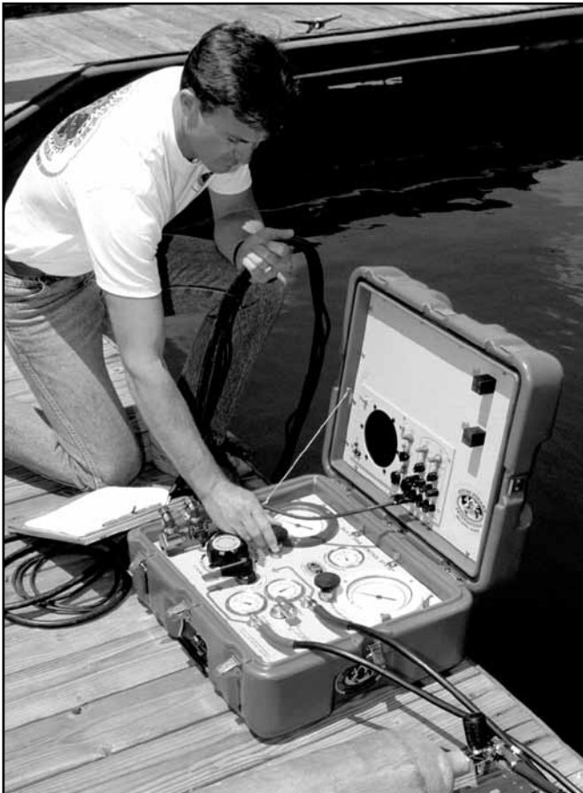
Figure 9 KMACS 5 operator taking a reading with the pneumo knob. The knob should be turned very slowly.
