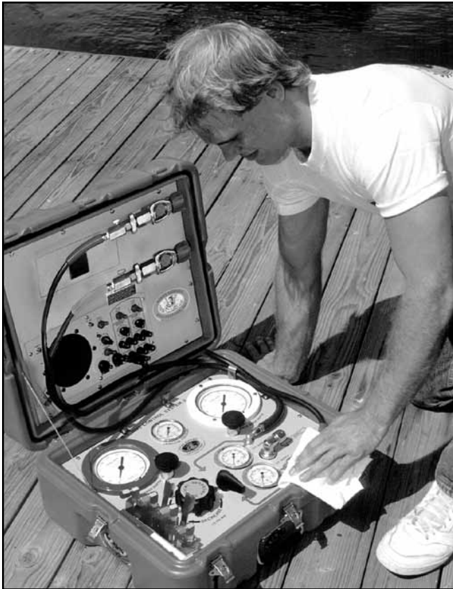
Figure 11 After each use the case, interior panels and high pressure hoses should be wiped down with a rag which has a small amount of Armor-All. Never spray cleaners directly on the KMACS 5.
