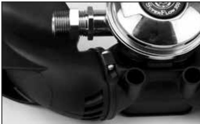
*To allow access to the two exhaust valves in the whisker wings, you must first remove the two whisker clamps that hold the whiskers on the exhaust main body. This is the starboard clamp.*
