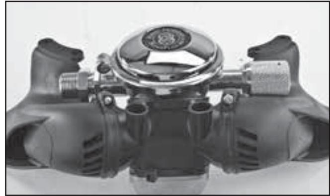
*To remove the Quad Valve or Tri-Valve exhaust from the helmet you must first cut the tie-wrap that secures the exhaust main body to the regulator.*
