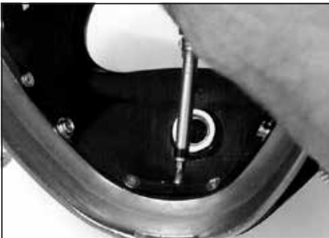
*To remove the water dump body you must remove the three screws inside the helmet shell.*
