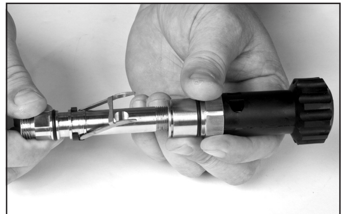
Separate the flex knob assembly from the main tube.
