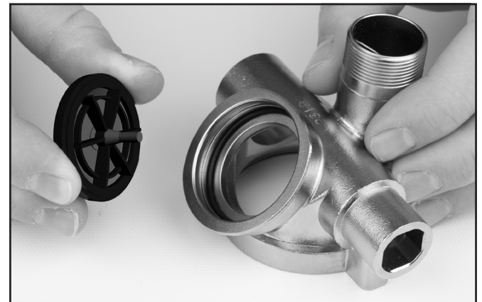
Install the O-ring and valve insert.
