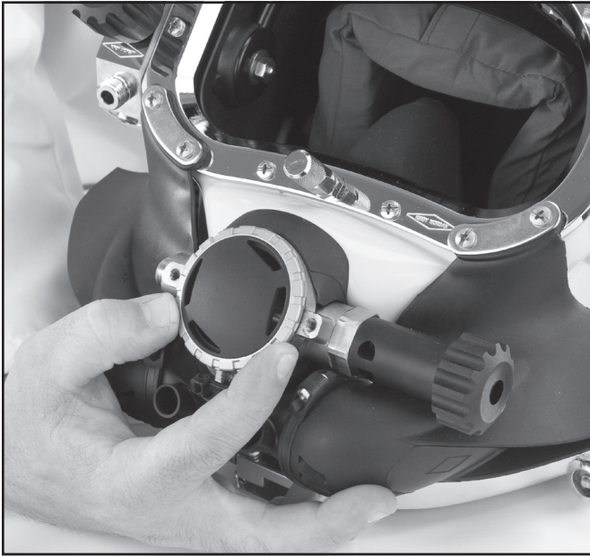
Unscrew the cover retaining ring and remove the cover.
