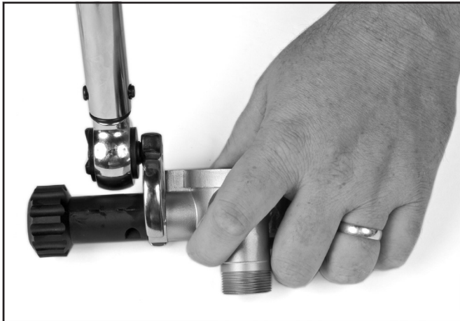
Torque the packing nut, see "Torque Specs" on page APNDX-19 for correct torque.
