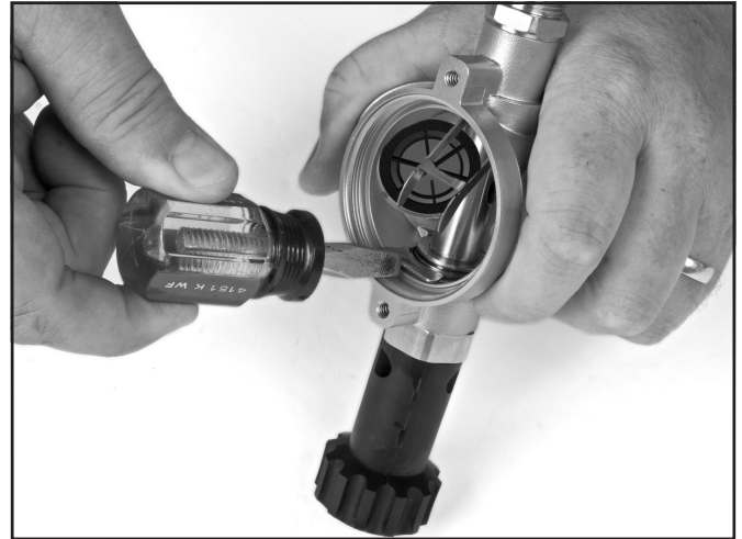
Make sure the lock clip fully engages the packing nut.
