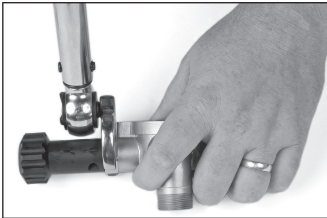
Unscrew the packing nut from the regulator body.
