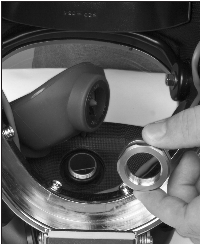
Install the regulator mount nut.
