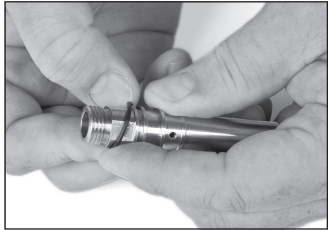
Install the O-ring on the main tube.
