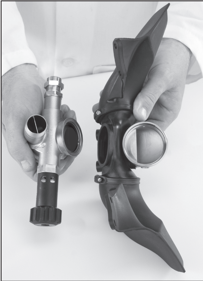
Separate the regulator from the Quad Valve™ exhaust whiskers.
